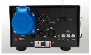
The Location Pro-Dim 10 is a versatile and portable single channel dimmer which can also be used for zero voltage switching of suitable loads. It features front panel mounted rotary level control, dimming/ switching selection rocker switch, mimic LED 'power connected' neon indicator and circuit breaker.
