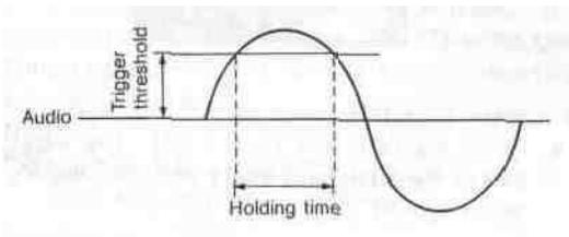
3. The A/V Synchronization holds the Strobe effect on for the period adjusted by the Effect Interval Timer (39).
