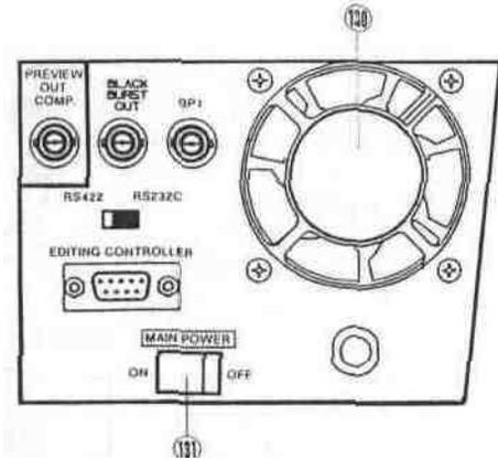
2. Press the OPERATE Button (1) on the operation panel. The unit is now in operation mode and the Cooling Fan (130) located on the rear panel starts to rotate. The LED's on the operation panel light up as shown if the RESET Switch (109) was already in the ON position.
