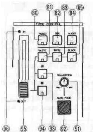
The VIDEO (80), DSK (82) and/or AUDIO (84) signals can fade out to one of the following : MATTE (81), WHITE (83), BLACK (85), A (93), or B (94) signal.
